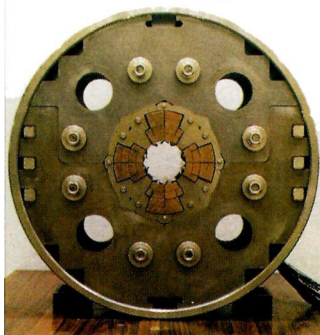
Japanese magnets for CERN's LHC – left, the cross-section of the short model, and right, the 1 m model assembly after the yoking process at the KEK laboratory.
